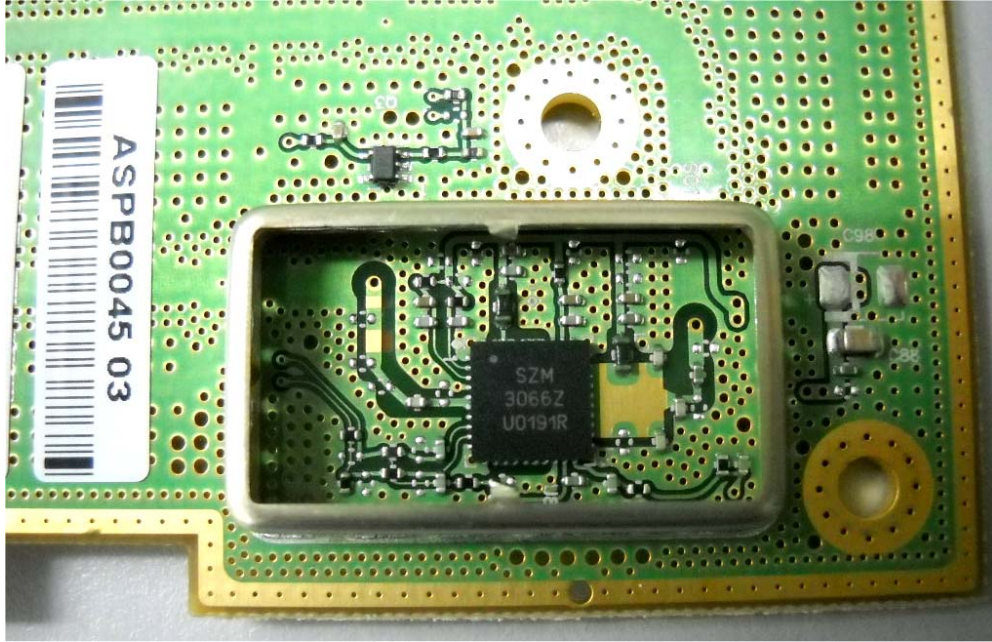
Photograph No.7 RF card front view with shield removed
