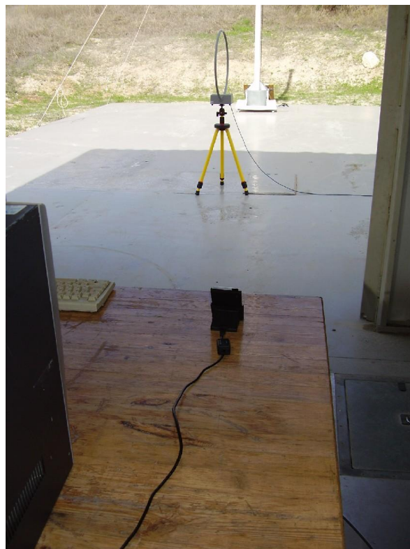
RE test setup on OATS.
