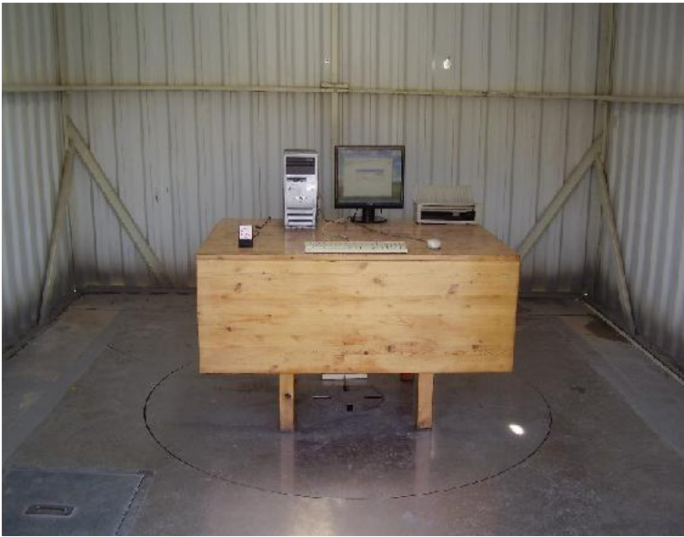
RE test setup on OATS.
