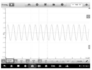
Figure 8-40 Sample Amplitude Setting Screen (AC 2.0V/div)
