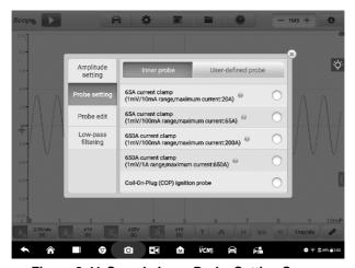
Figure 8-41 Sample Inner Probe Setting Screen
