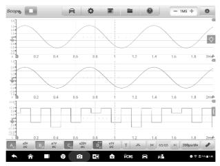
Figure 8-20 Sample Triple Window Screen
