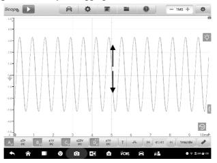
Figure 8-33 Sample Dragging Waveform or Moving Screen
