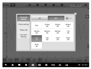
Figure 8-39 Sample Amplitude Setting Screen (AC 2.0V/div)
