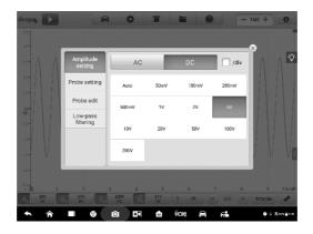
Figure 8-37 Channel Setting Dialog Box Screen
