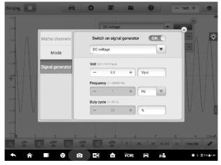
Figure 8-16 Sample Signal Generator Settings Screen
