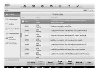
Figure 4-30 Sample DTC & FFD Screen
