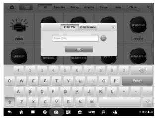
Figure 4-5 Sample Manual VIN Input
