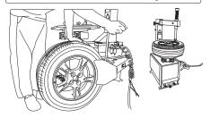
3 -Dismounting the sensor----Remove the fastening screw and the sensor from the valve stem with a screwdriver, and then loosen the
