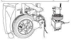
3 Dismounting the sensor Remove the fastening screw and the sensor from the valve stem with a screwdriver, and then loosen the nut to remove the valve.
