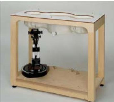
The SAM twin phantom is a fiberglass shell phantom with 2mm shell thickness (except the ear region where shell thickness increases to 6mm). It has three measurement areas:
