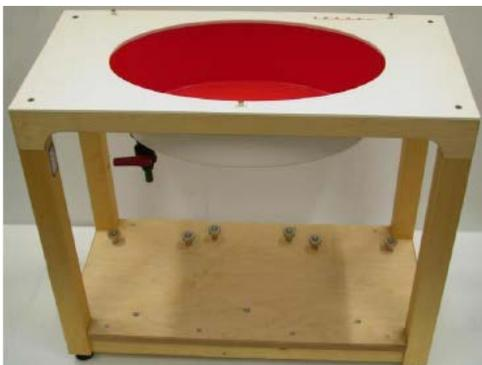
The ELI4 phantom is intended for compliance testing of handheld and body-mounted wireless devices in the frequency range of 30 MHz to 6 GHz. ELI4 is fully compatible with standard and all known tissue simulating liquids.
