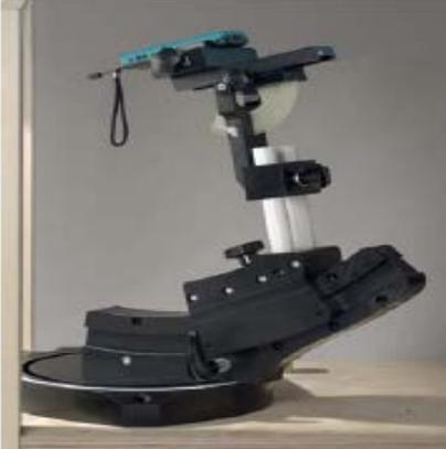
The DASY device holder is designed to cope with different positions given in the standard. It has two scales for the device rotation (with respect to the body axis) and the device inclination (with respect to the line between the ear reference points). The rotation centers for both scales is the ear reference point (ERP). Thus the device needs no repositioning when changing the angles.
