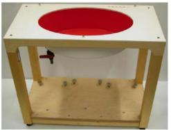
The ELI4 phantom is intended for compliance testing of handheld and body-mounted wireless devices in the frequency range of 30 MHz to 6 GHz. ELI4 is fully compatible with standard and all known tissue simulating liquids. Shell Thickness:  $2 \pm 0.2$  mm (sagging: <1%) Filling Volume: Approx. 30 liters Dimensions: Major ellipse axis: 600 mm Minor axis: 400 mm
