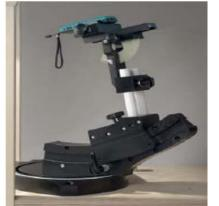
The DASY device holder is designed to cope with different positions given in the standard. It has two scales for the device rotation (with respect to the body axis) and the device inclination (with respect to the line between the ear reference points). The rotation centers for both scales is the ear reference point (ERP). Thus the device needs no repositioning when changing the angles.
