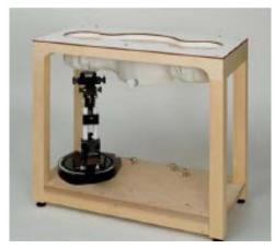
The light beam switch allows automatic "tooling" of the probe. During the process, the actual position of the probe tip with respect to the robot arm is measured, as well as the probe length and the horizontal probe offset. The software then corrects all movements, such that the robot coordinates are valid for the probe tip. The repeatability of this process is better than 0.1 mm.
