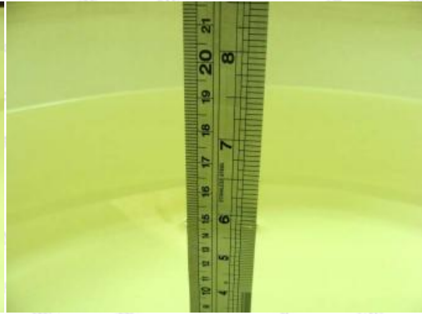
Photo of Liquid Height for Body SAR
