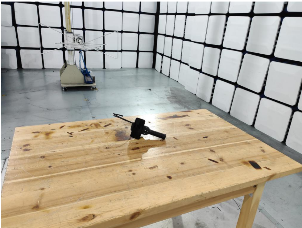
Photo of Radiation Emission Test
