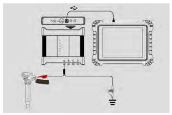
Figure 9-1 Sample Connection Diagram
