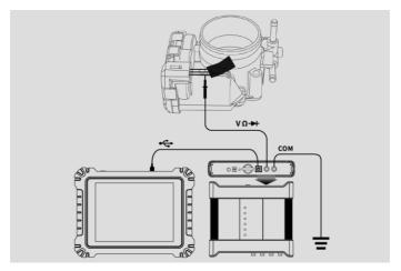
Figure 9-1 Sample Connection Diagram
