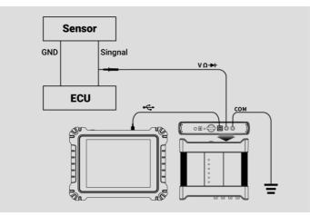
Figure 9-16 Sample Triangle Waveform Connection Diagram
