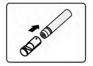
2. Slip the end of the accessory over the imager head and then fix the accessory.
