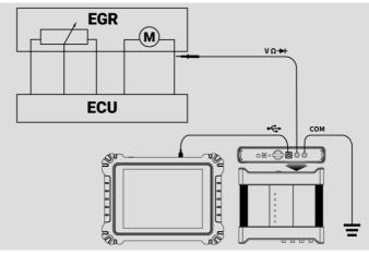
Figure 9-12 Sample Duty Cycle Connection Diagram
