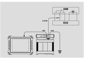
Figure 9-11 Sample DC Voltage Connection Diagram
