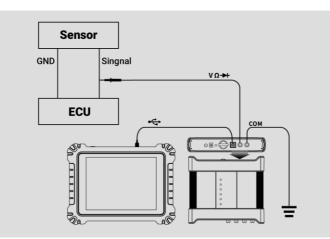
Figure 9-17 Sample Arbitrary Waveform Connection Diagram
