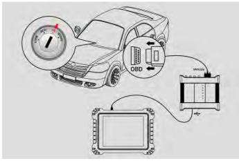
Figure 9-1 Sample Connection Diagram
