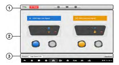
Figure 9-4 Sample OBD Communication Line Inspection Menu Screen
