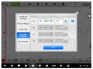
Figure 9-47 Sample Lowpass Filtering Screen
