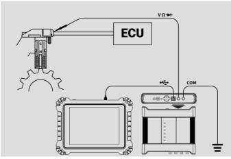
Figure 9-14 Sample Sinusoid Connection Diagram
