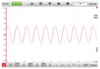
Figure 9-40 Sample Amplitude Setting Screen (AC 2.0V/div)
