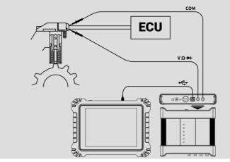
Figure 9-15 Sample X+Y Waveform Connection Diagram
