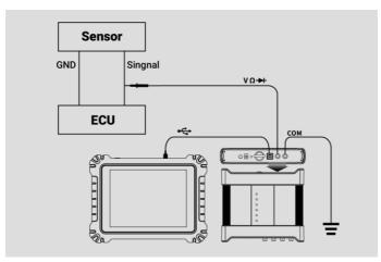
Figure 9-1 Sample Connection Diagram
