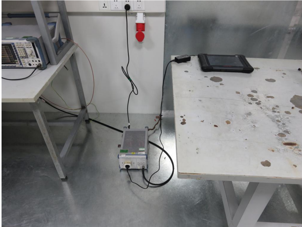
Photo of Conducted Emission Measurement
