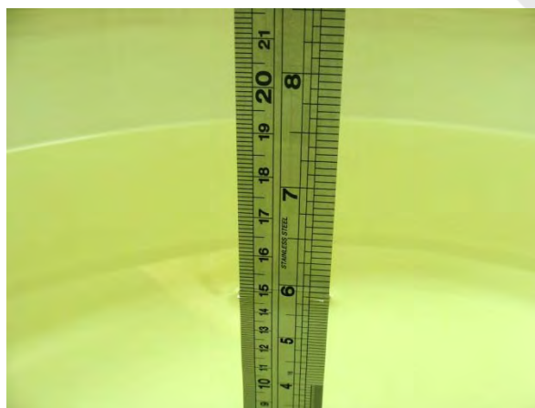
Photo of Liquid Height for Body SAR
