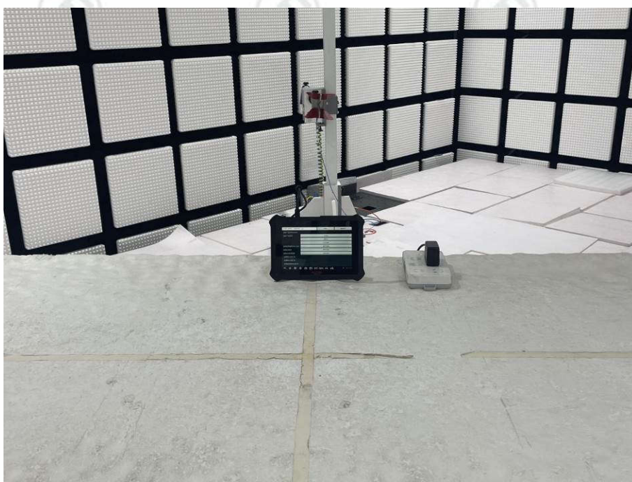
Radiated spurious emission Test Setup-2(Above 1GHz)
