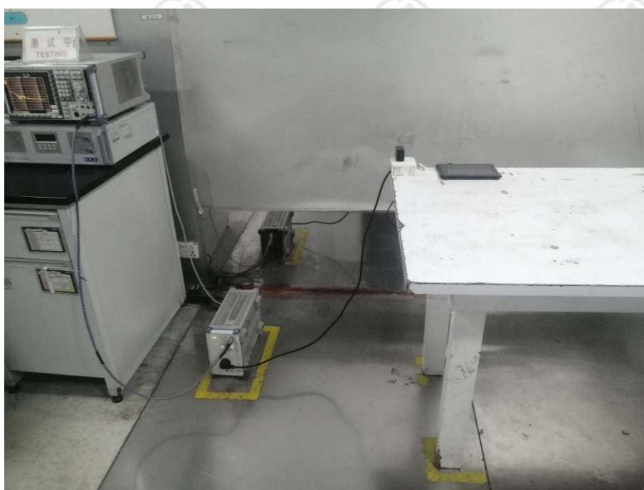
Conducted Emissions Test Setup
