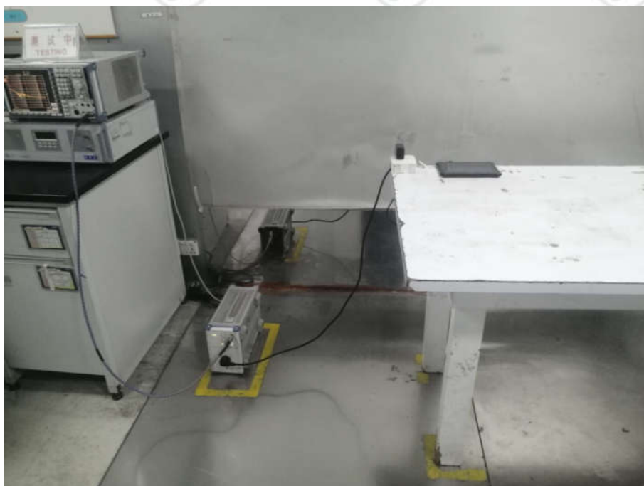
Conducted Emissions Test Setup
