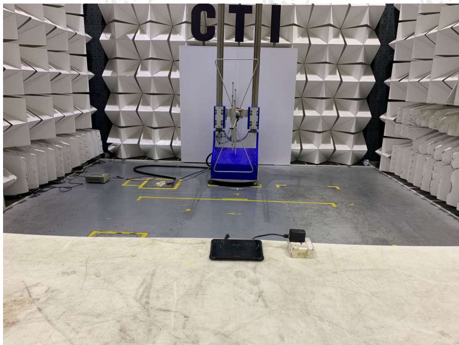
Radiated spurious emission Test Setup-3(Below 1GHz)
