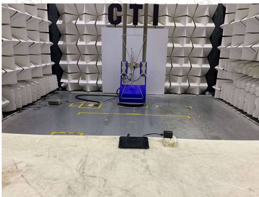
Radiated spurious emission Test Setup-2(Below 1GHz)
