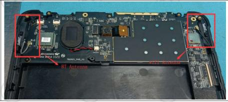
The antenna is integrated on the main PCB and no consideration of replacement. The best case gain of the antenna is 4.21dBi.
