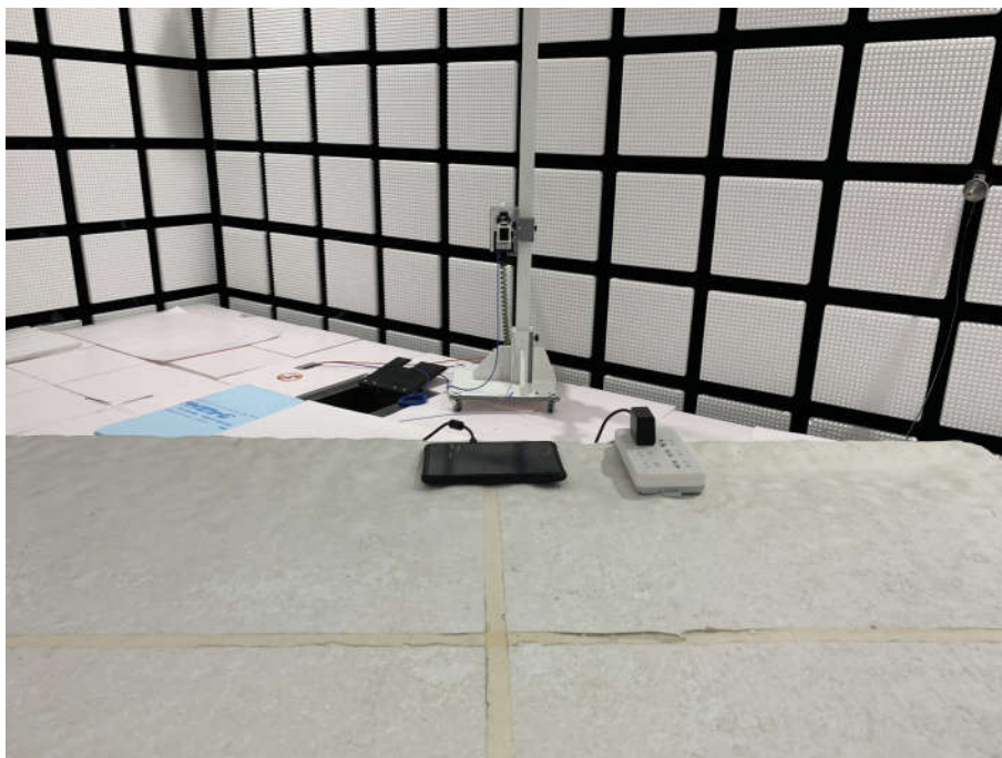
Radiated spurious emission Test Setup-4(Above 18GHz)
