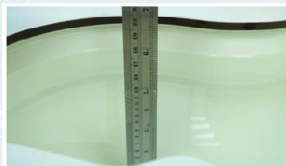
Photo of Liquid Height for Head SAR
