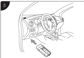
Insert the Vehicle Data Connector on the MaxiVCI V200 into the vehicle's DLC, which is generally located under the vehicle dashboard.
