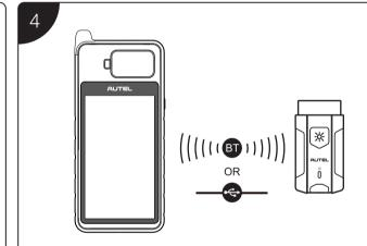
Turn the vehicle ignition to the ON position and pair the KM100 with the MaxiVCI V200 via Bluetooth or connect via supplied USB cable to establish a communication link. Your key tool is now ready for use.
