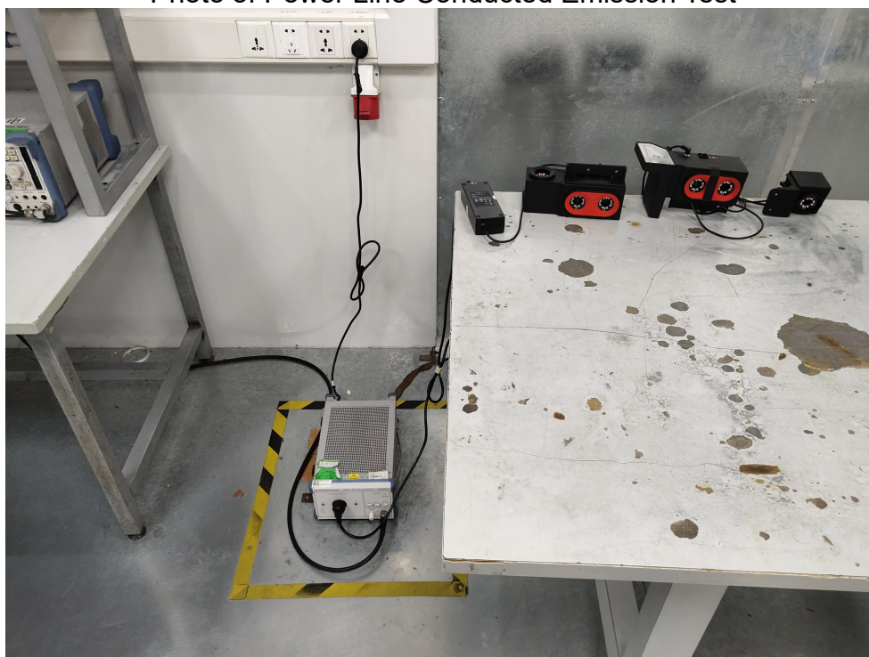
FCC ID: WQ8IA800-CAM Photo of Power Line Conducted Emission Test
