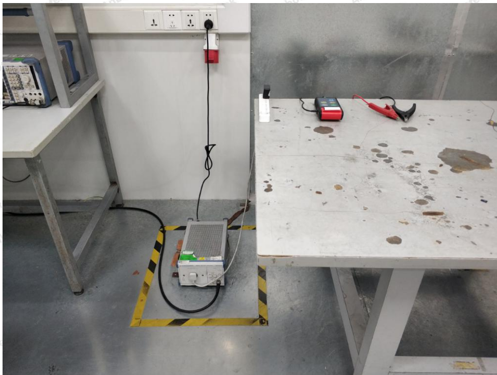
Photo of Conducted Emission Measurement
