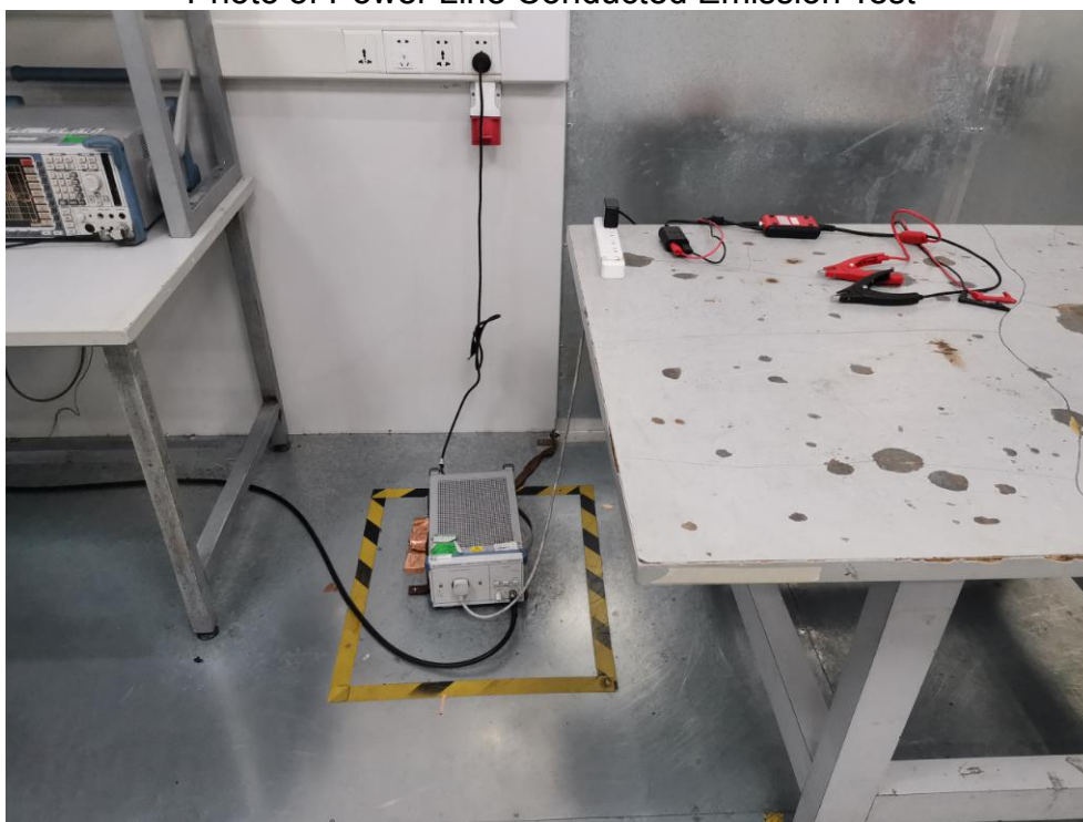
FCC ID: WQ8BATS-BT508 Photo of Power Line Conducted Emission Test
