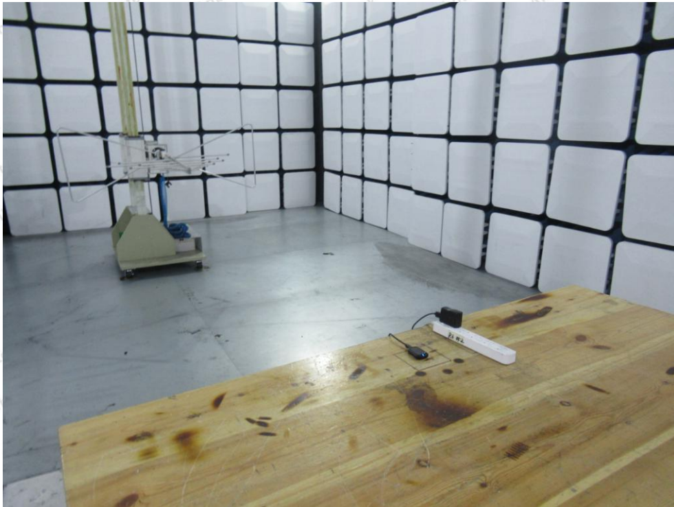
Photo of Radiation Emission Test
