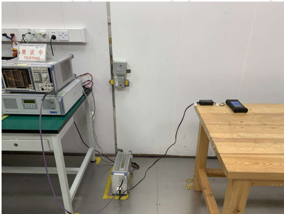
Conducted Emissions Test Setup
