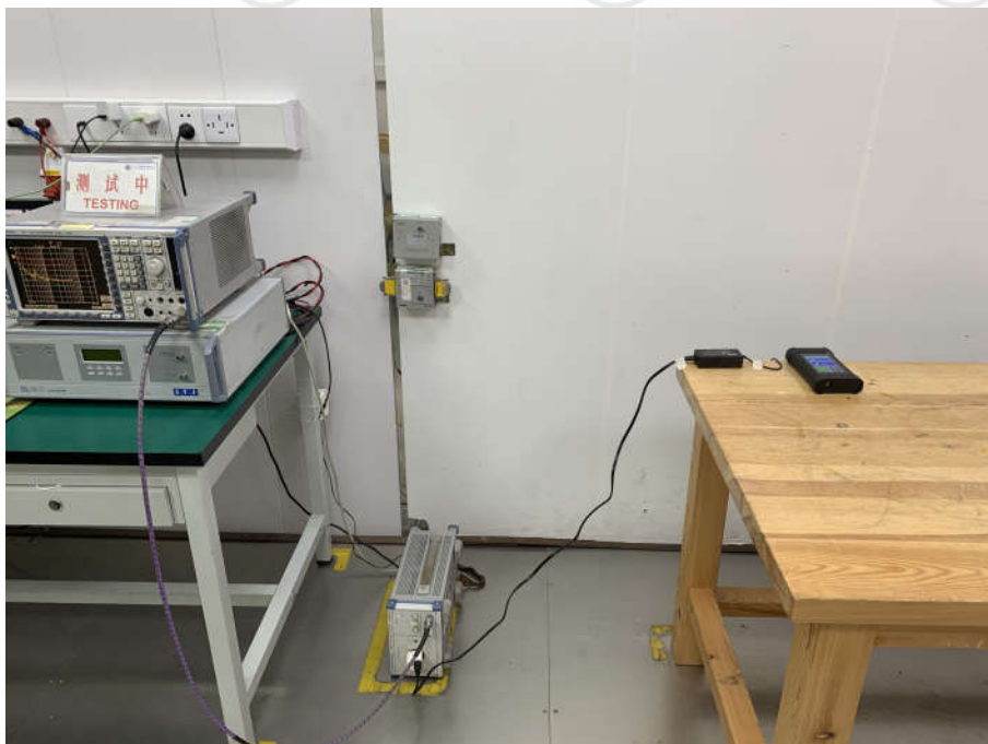
Conducted Emissions Test Setup
