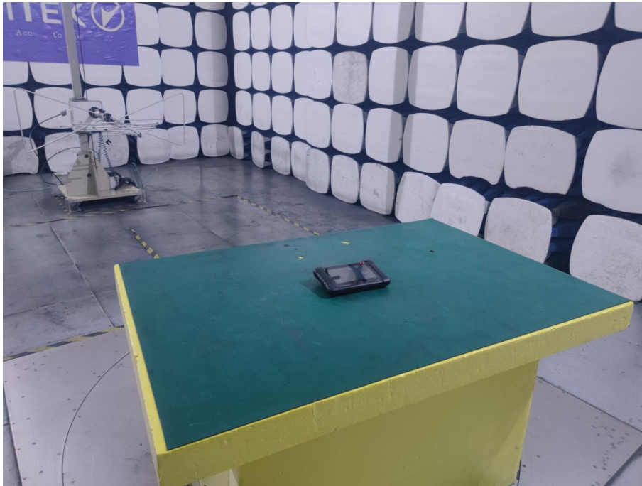
Spurious Emission Test Setup (Above 1GHz)
