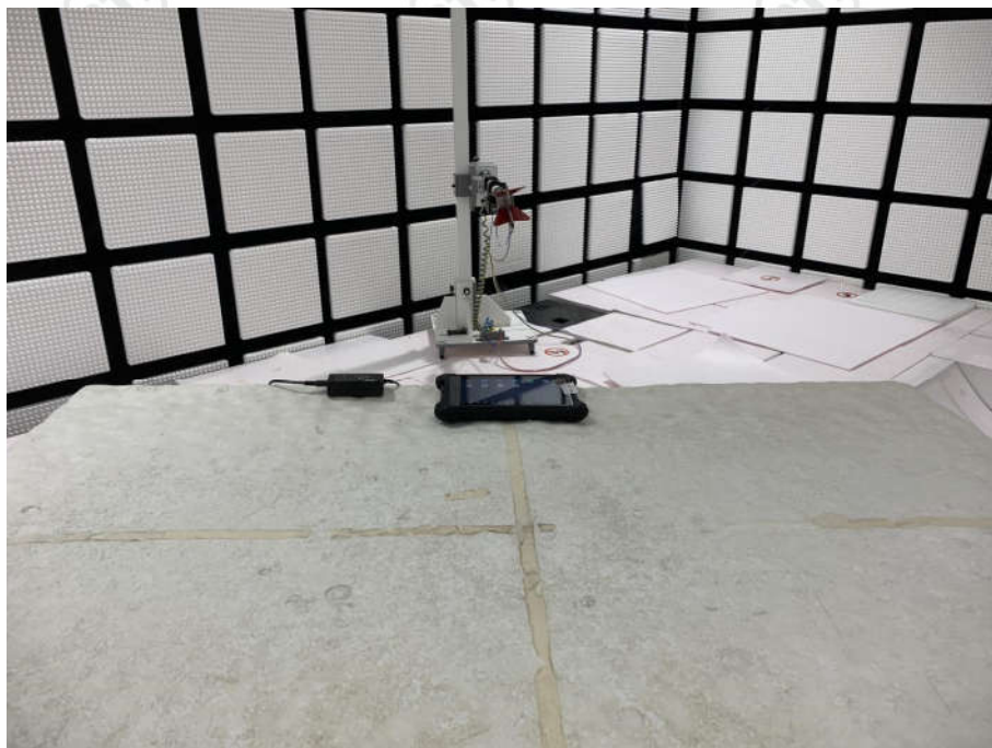
Radiated spurious emission Test Setup-2(Above 1GHz)
