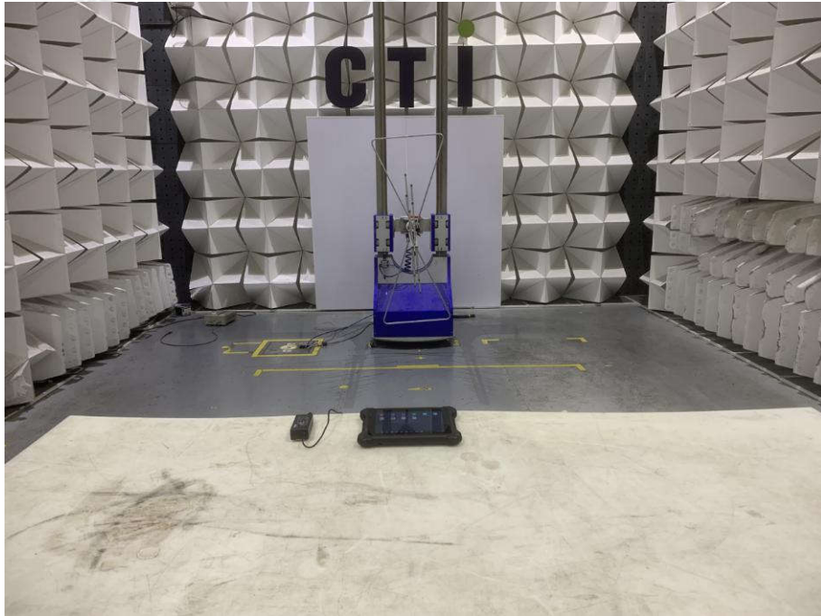
Radiated spurious emission Test Setup-1(Below 1GHz)
