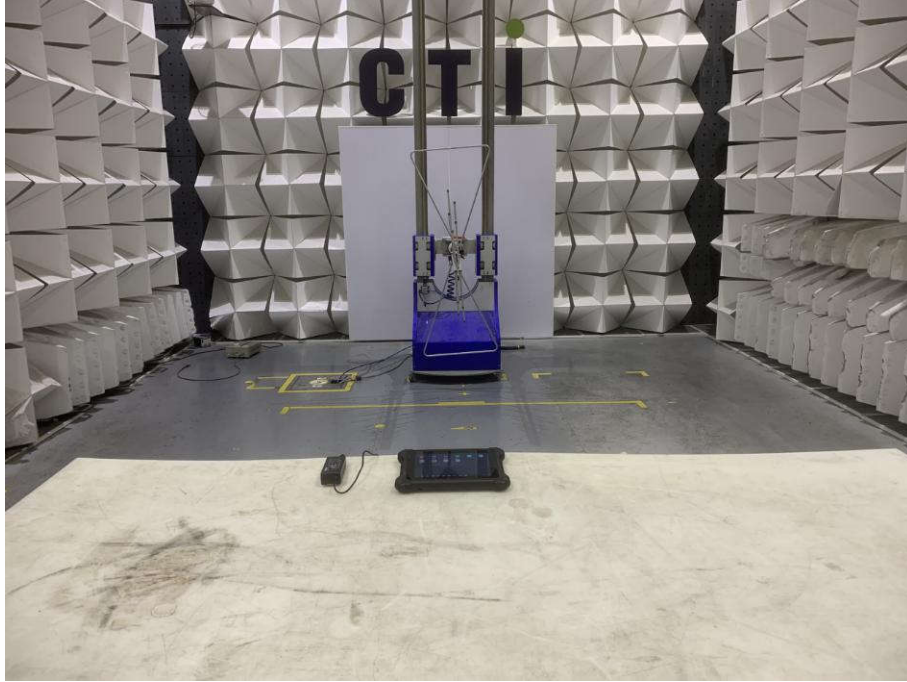
Radiated spurious emission Test Setup-1(Below 1GHz)
