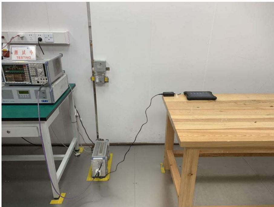
Conducted Emissions Test Setup
