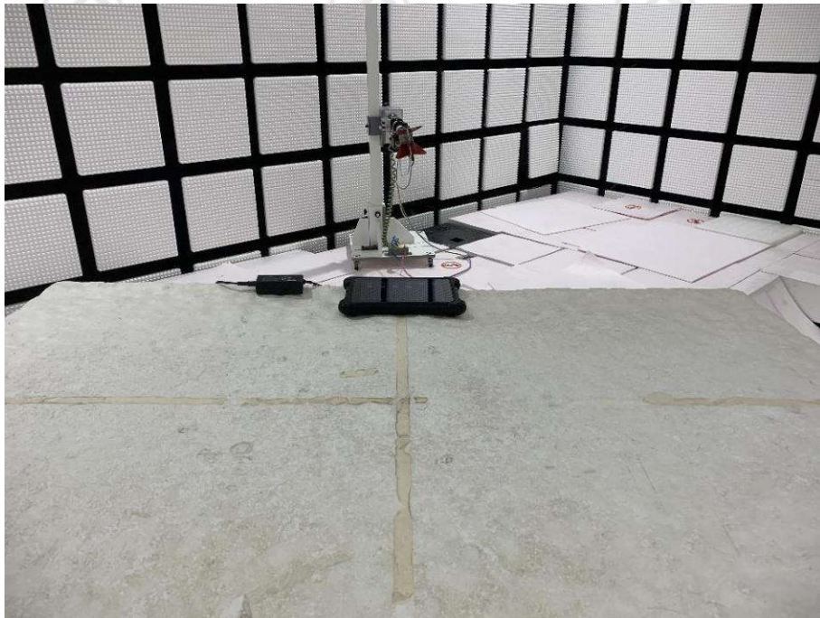
Radiated spurious emission Test Setup-2(Above 1GHz)
