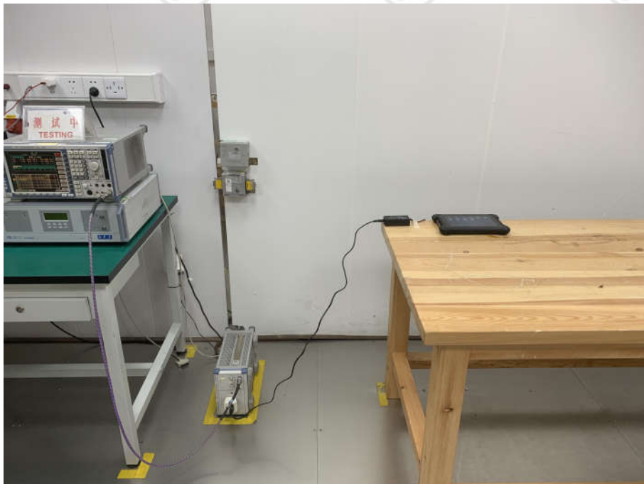
Conducted Emissions Test Setup
