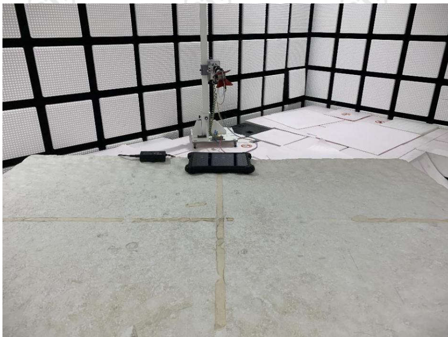
Radiated spurious emission Test Setup-2(Above 1GHz)
