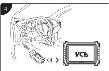
• When the MaxiVCI V200 is properly connected to the vehicle and the tablet, the VCI status button on the bottom bar of the screen will display a green badge with a check mark at the corner indicating the tablet is ready to start vehicle diagnosis. FCC STATEMENT :
