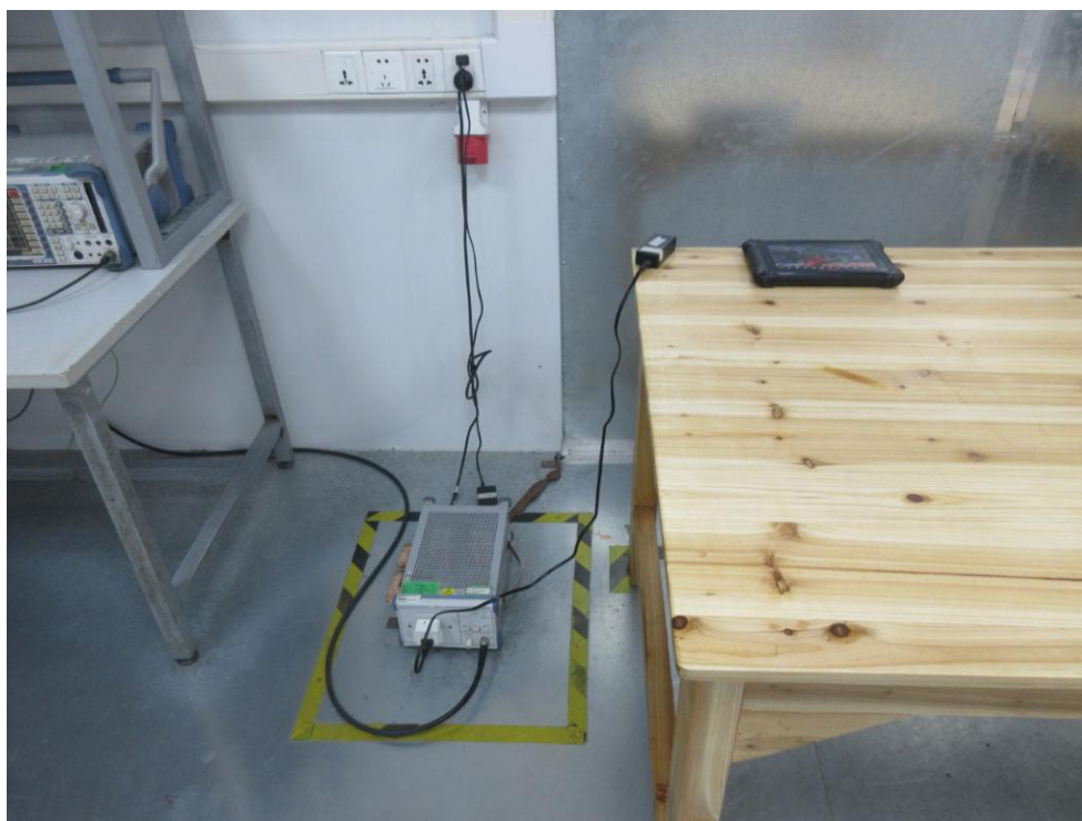
Photo of Conducted Emission Measurement
