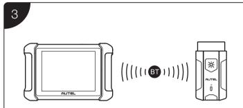
Pair up the Display Tablet with the MaxiVCI V200 via wireless BT to establish a communication link.
