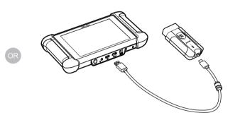
Or, connect the Display Tablet and MaxiVCI V200 using the USB cable.
