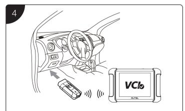
When the MaxiVCI V200 is properly connected to the vehicle and the Display Tablet, the VCI status button at the bottom bar on the display screen shows a green check mark at the corner. This indicates the platform is ready to start vehicle diagnosis.
