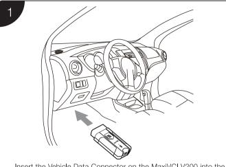
Insert the Vehicle Data Connector on the MaxiVCI V200 into the vehicle's DLC, which is generally located under the vehicle dash.
