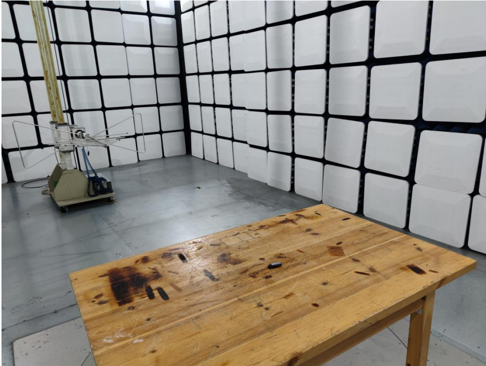
Photo of Radiation Emission Test
