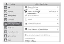
Tap the ADAS & Aligner Settings option on the left column. Tap the Camera Connection setting to display the Wi-Fi connection screen.
