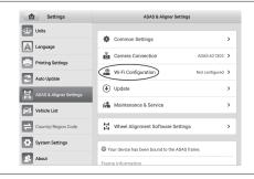
Tap **Settings > ADAS & Aligner Settings > Wi-Fi Configuration** to enter the Wi-Fi configuration screen.
