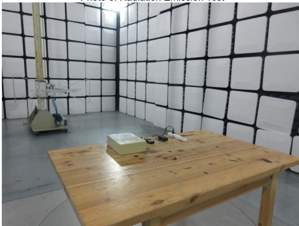
Photo of Radiation Emission Test
