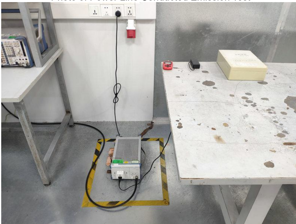
FCC ID: WQ8-DR2013 Photo of Power Line Conducted Emission Test
