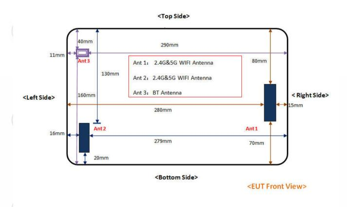
Note:1)Per KDB 616217, because the diagonal Length is >200mm, it is considered a "tablet" device and need to test 0mm 1g Body SAR.
