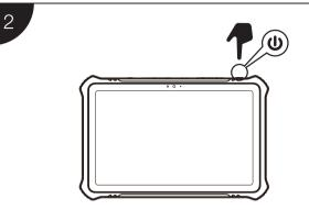
• Long press the **Power/Lock** button to power up the diagnostics tablet. Ensure the tablet has a charged battery or is connected to the supplied DC power supply.
