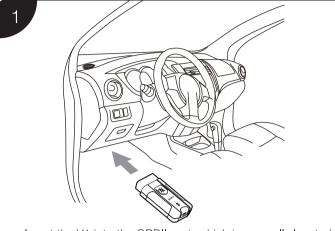
• Insert the V1 into the OBDII port, which is generally located under the vehicle dashboard.
