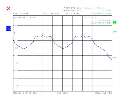
Test mode: π/4DQPSK Test channel: Lowest
