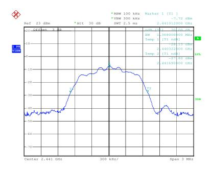
Test mode: π/4DQPSK Test channel: Highest
