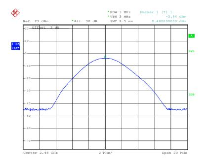
Test mode: π/4DQPSK Test channel: Lowest
