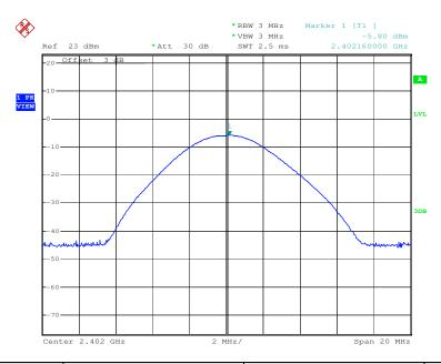
Test mode: GFSK Test channel: Middle
