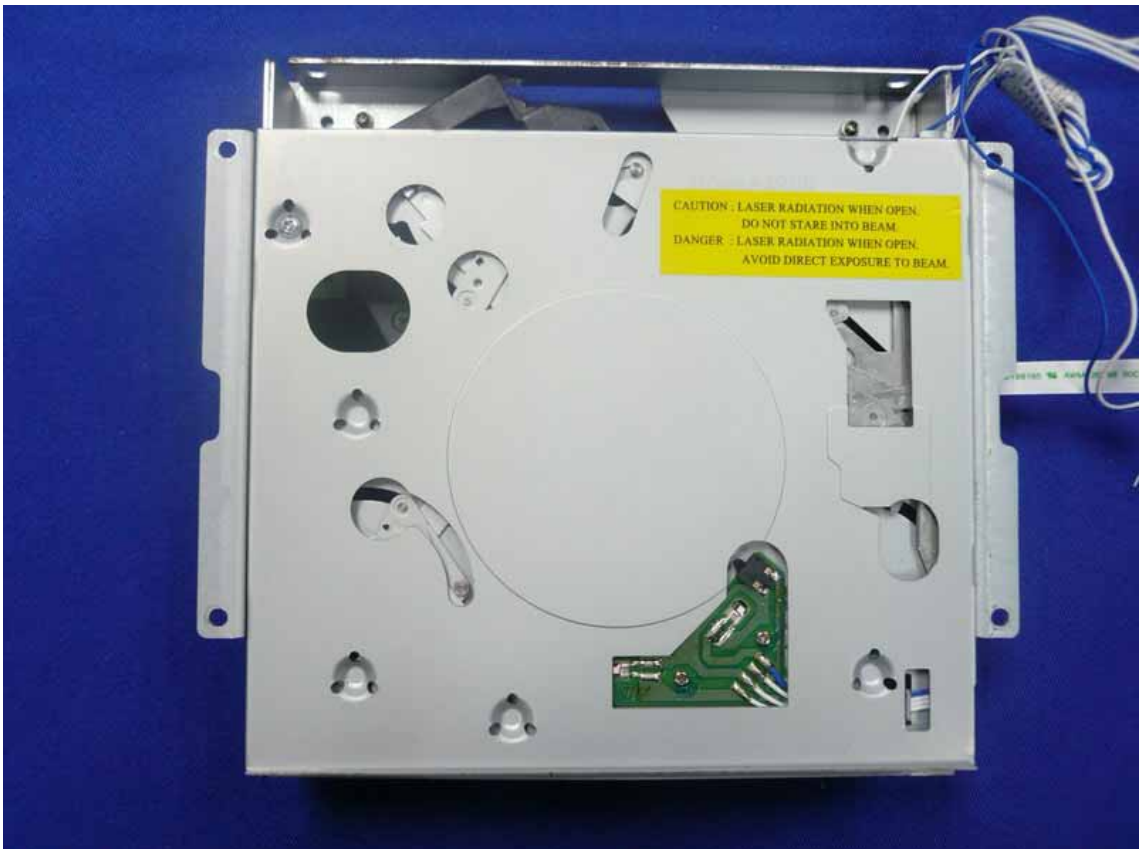
Figure 38 Inside of the External functional module
