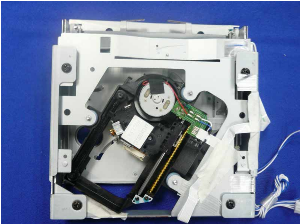
Figure 37 Inside of the External functional module
