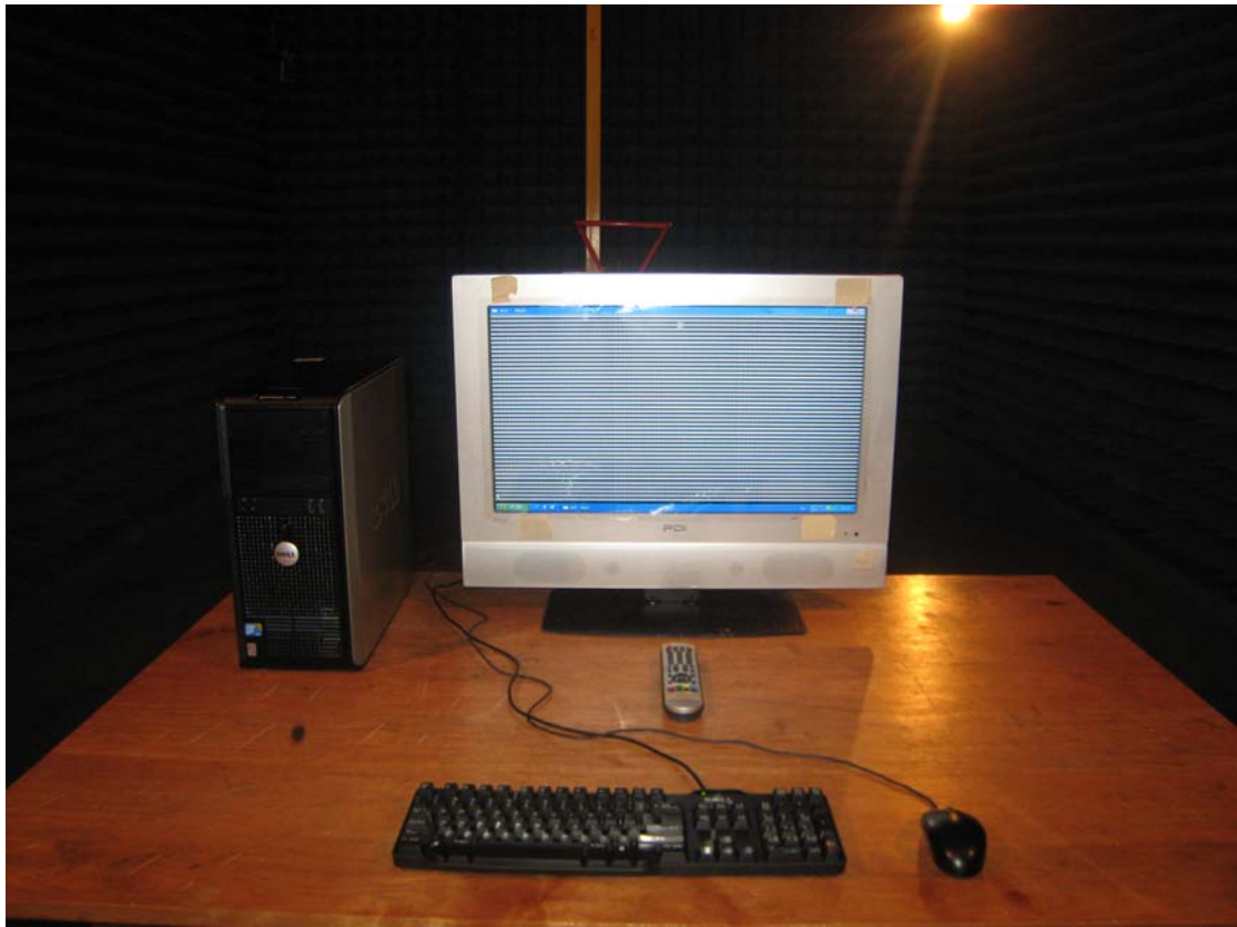
Test photo of radiated emission (30MHz-1000MHz)
