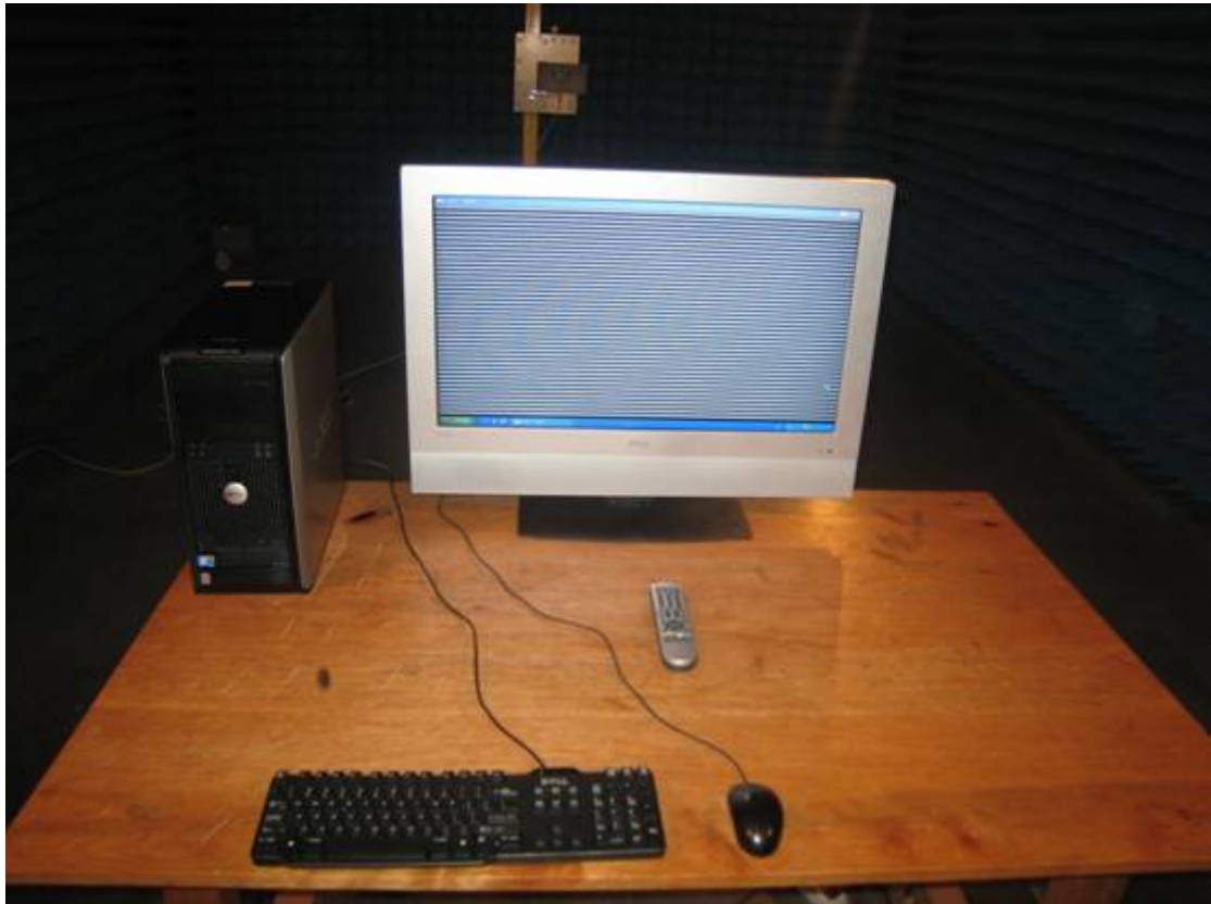
Test photo of radiated emission (1000MHz-5000MHz)
