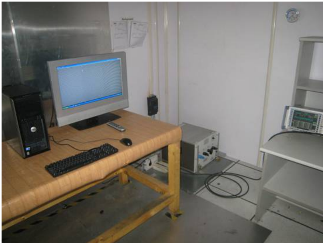
Test photo of Conducted emission
