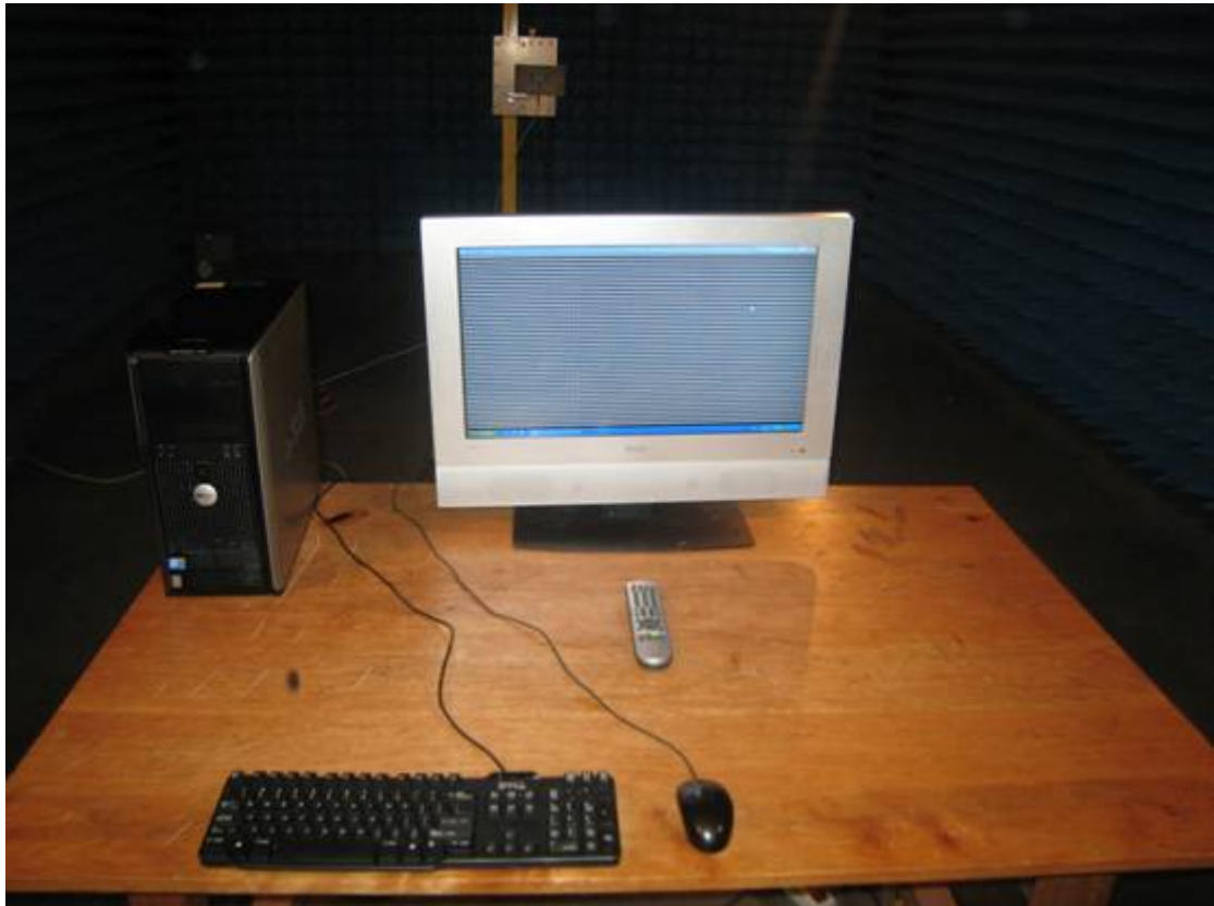
Test photo of radiated emission (1000MHz-5000MHz)
