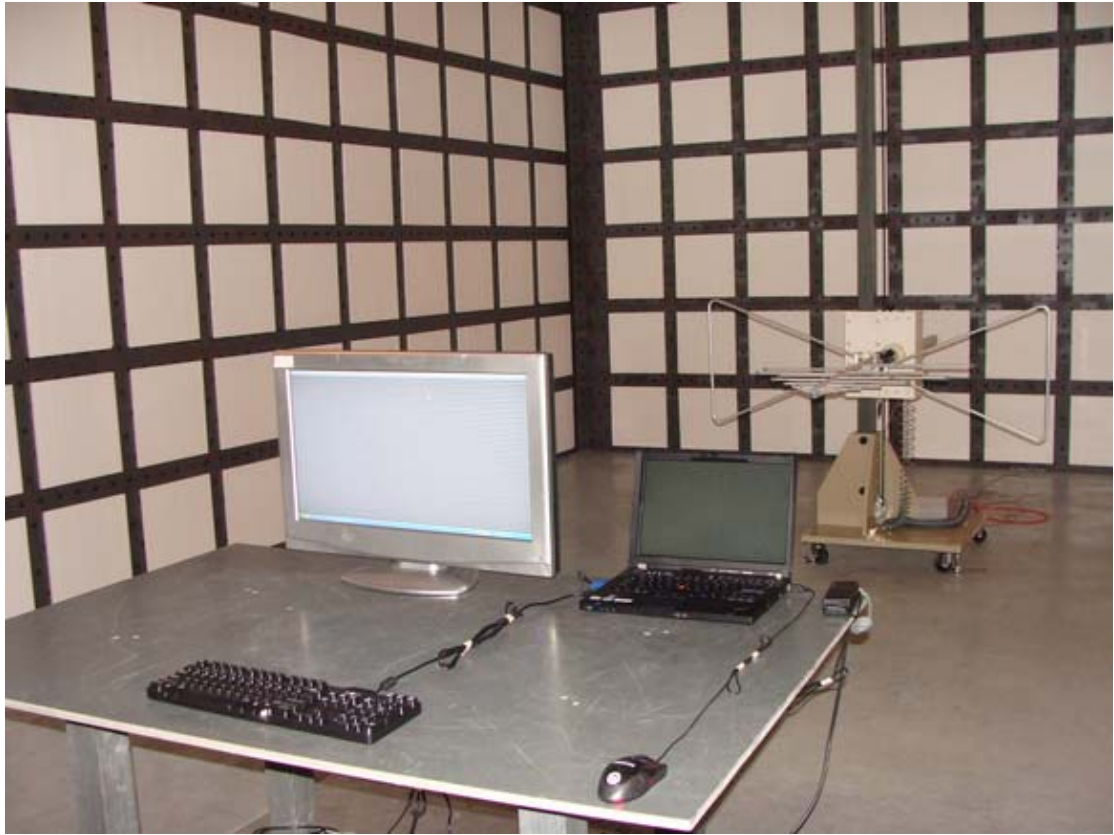
Radiated emission test view
