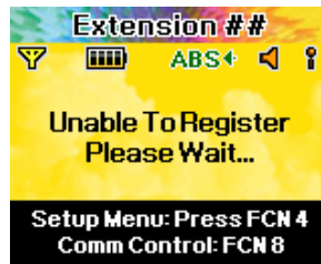
Display #5 - Idle mode (Unlocked, Disconnected)
