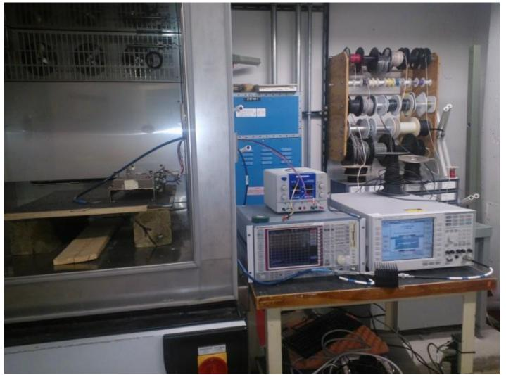
\* antenna port measurements for power and bandwidth were done outside of the chamber, but in the same configuration / connection setup as above.
