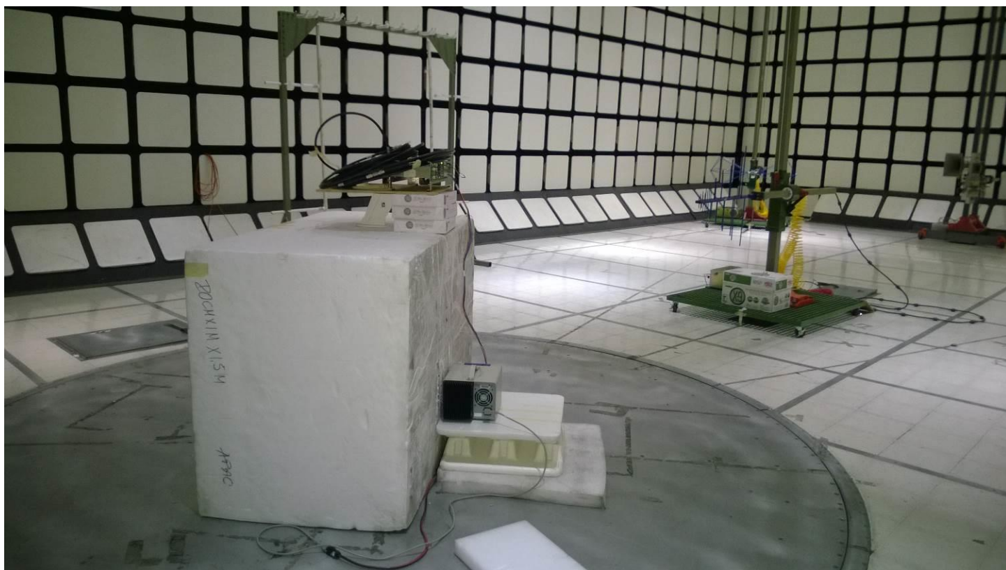
Antenna Configured in Z-Axis Position
