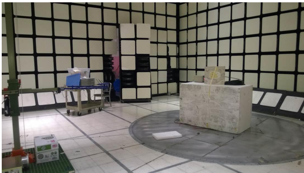
Antenna Configured in X-Axis Position
