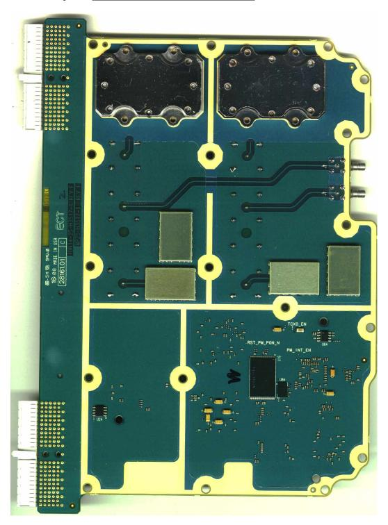
Photo Description: Bigsky Aircard circuit board – Side 1 with shields removed
