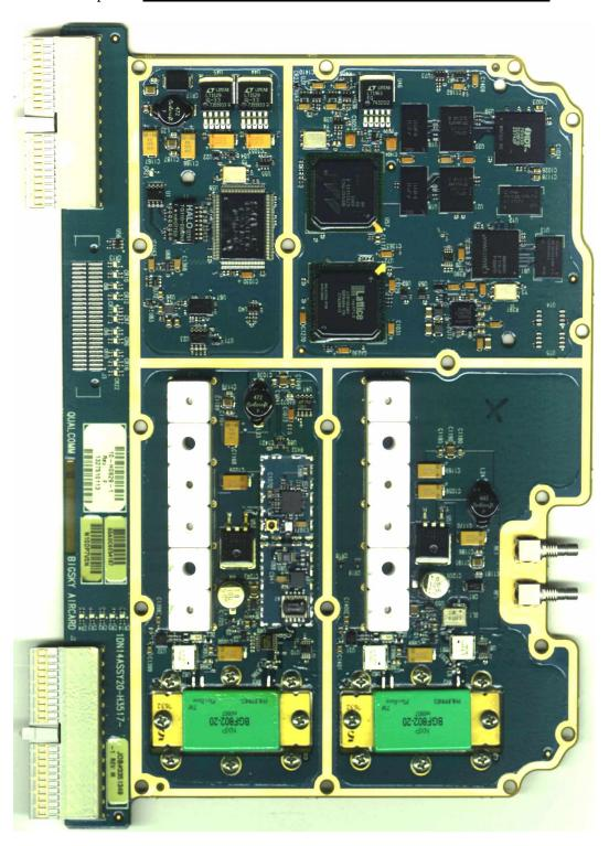
Photo Description: Bigsky Aircard circuit board – Side 2 with shields removed
