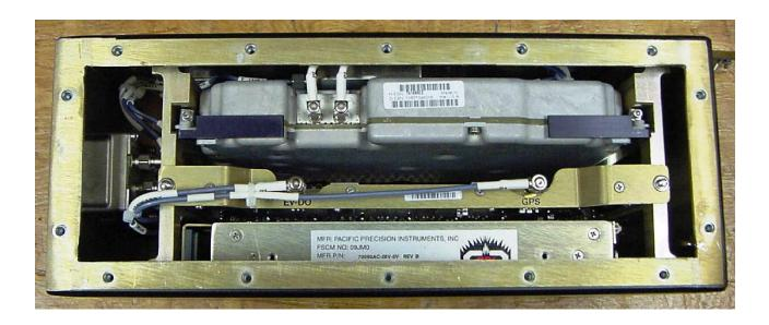
Photo Description: AACU with Bigsky Aircard module removed
